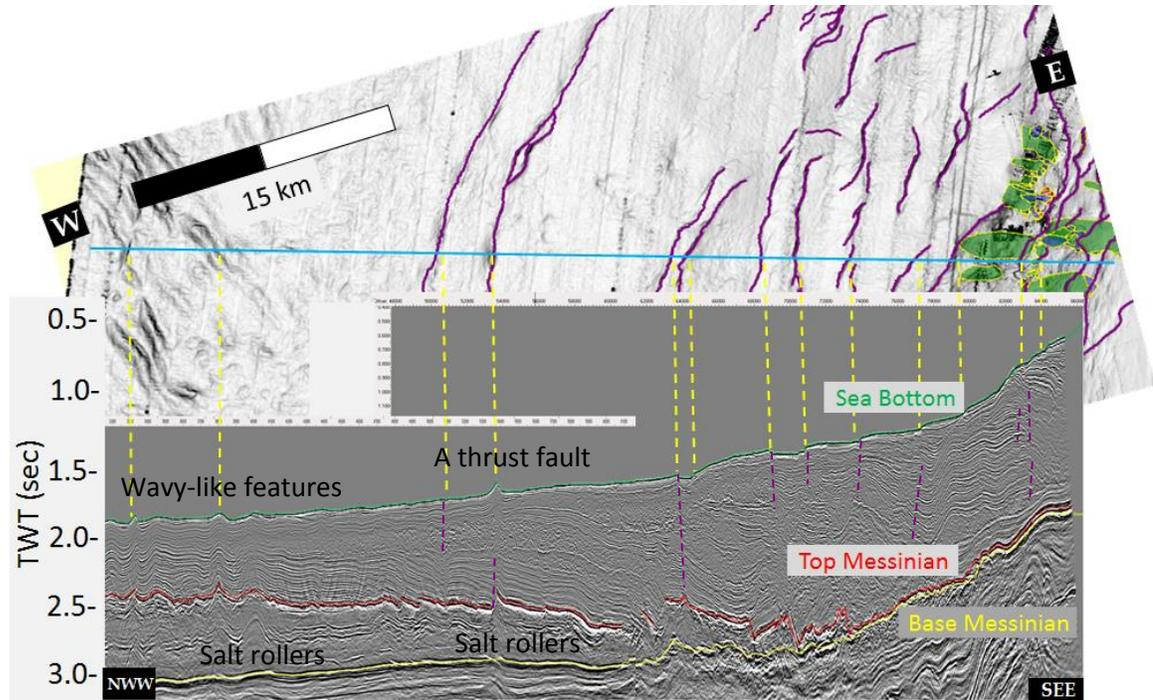
**Figure 26:** A seismic cross section of the studied area (for location see Fig. 11). Sea bottom, top Messinian and base Messinian horizons are marked in green, red and yellow respectively.
