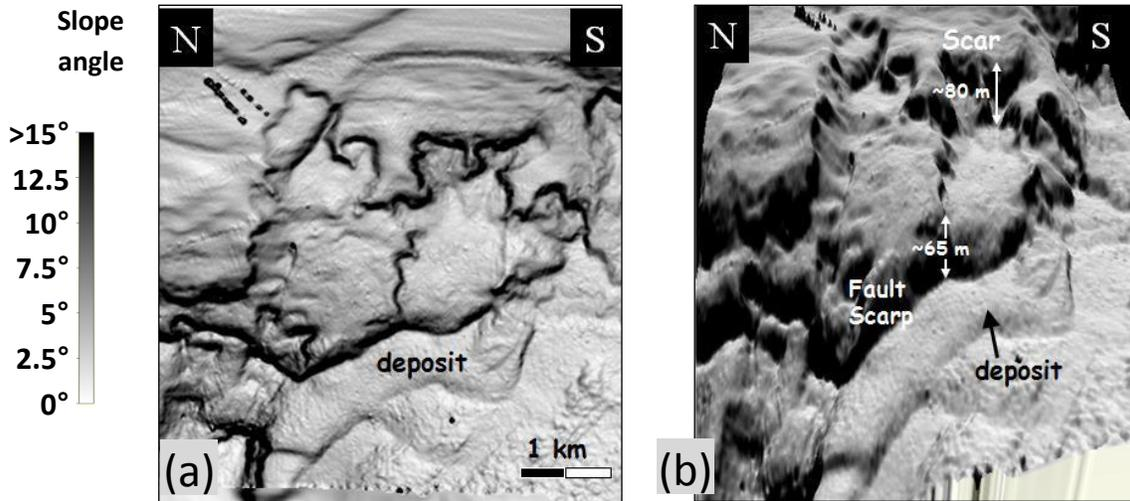
Figure 13: A map view (a) and a perspective view (b) of soil slump slide, characteristic of the northern part of the open slope (location is in Fig. 11).
