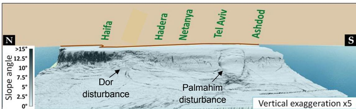
Figure 6: A perspective view of the studied area looking eastwards (from the basin towards the land). A Steep slope cut by canyons in the north, gradually changes southward to moderate open-slope with landslides.
