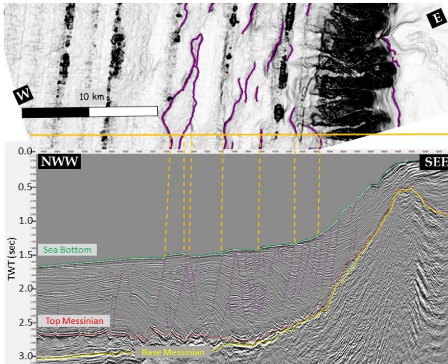
**Figure 25:** Faults in map view and in seismic cross section are marked in purple (for location see Fig. 11). Sea bottom, top Messinian and base Messinian horizons are marked in green, red and yellow respectively.
