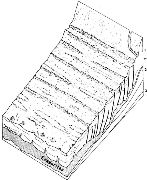
Figure 7: A Diagram showing faults and listric faults rooted at the Messinian evaporites (Almagor & Garfunkel, 1979). Vertical exaggeration = ~ 12 X.
