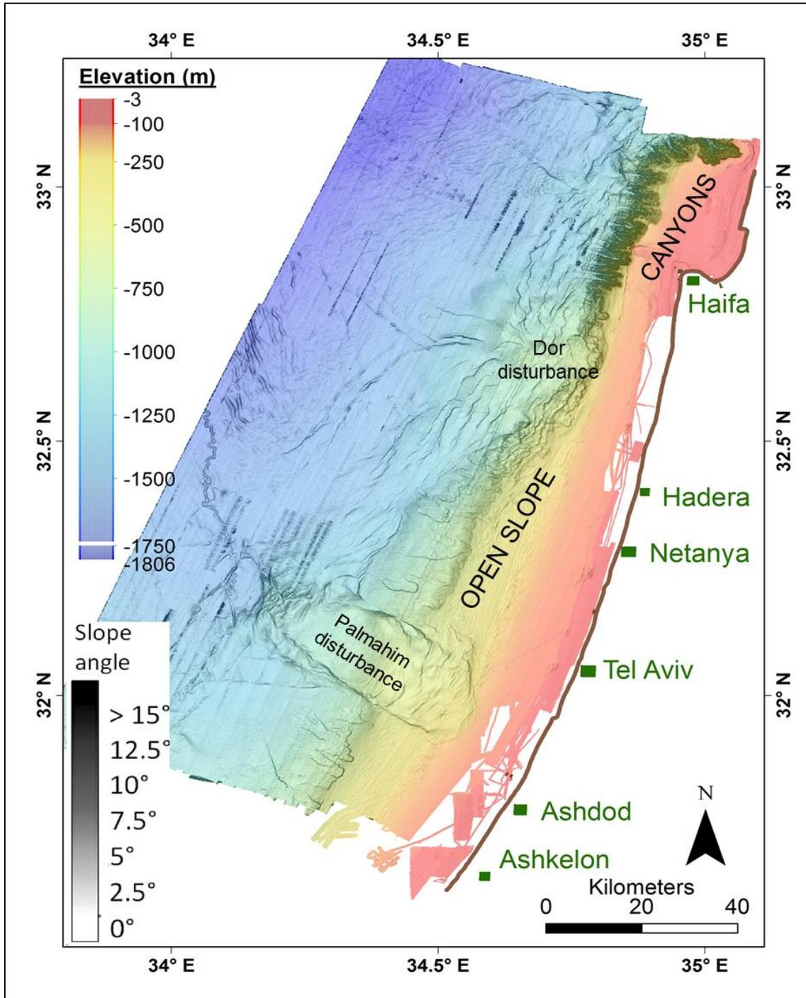
Figure 2: A map showing the bathymetry and the slope angle of the studied area (Sade, 2007; Sade et al., 2007; Tibor et al., 2013).
