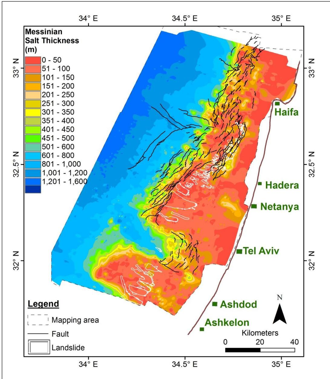
**Figure 28:** Landslides and faults shown on top of an isopach map of the Messinian salt.
