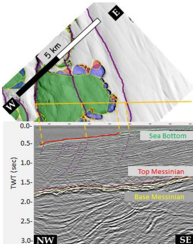
**Figure 18:** A map view and in a seismic cross section showing a landslide disrupted by faults, typical of the northern part of the studied slope. The landslide location is shown in Fig. 11. Sea bottom, top Messinian and base Messinian horizons are marked in green, red and yellow respectively. Landslide is marked in red in the section. Listric and normal faults are marked in purple in the seismic section. A few of them create a step on the bathymetry (marked in purple in the map view).
