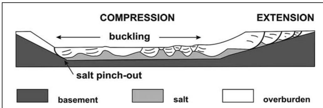
Figure 8: Model of gravity gliding (Letouzey et al., 1995 *in*: Gradmann et al., 2005). Gravity driven faulting above a viscous salt layer on the slope yields extension and basinward movement. This ceases where the salt layer pinches out and the overburden gets buckled and folded, showing a compressional stress regime.
