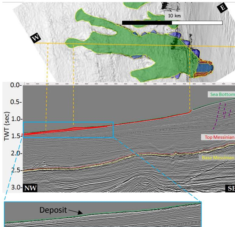
**Figure. 17:** Southern landslide in map view and in seismic cross section. Its location is in fig. 11. Sea bottom, top Messinian and base Messinian horizons are marked in green, red and yellow respectively. Faults are marked in purple and the landslide with its deposit is marked in red in the seismic section. In the small figure: the material inside the landslide's deposit seems granular and chaotic and it is elevated from the sea floor.
